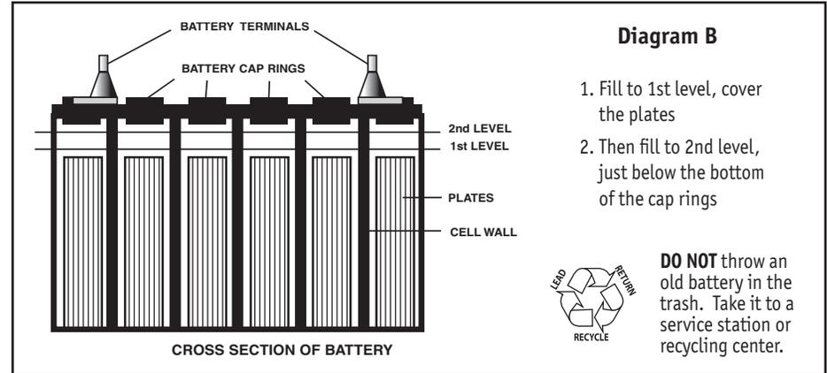
of the battery to a level just covering the battery plates, and then go back and top off each cell equally. It is important to have all the cells filled equally or the battery will not operate properly. The acid should reach a level about ¼" below the cap ring as shown in the diagram above. **DO NOT OVERFILL THE BATTERY.** (Diagram B)
