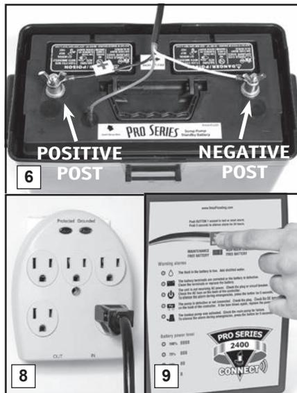
9. If any of the alarms are sounding, press the RED button on the front of the control panel for one (1) second.
