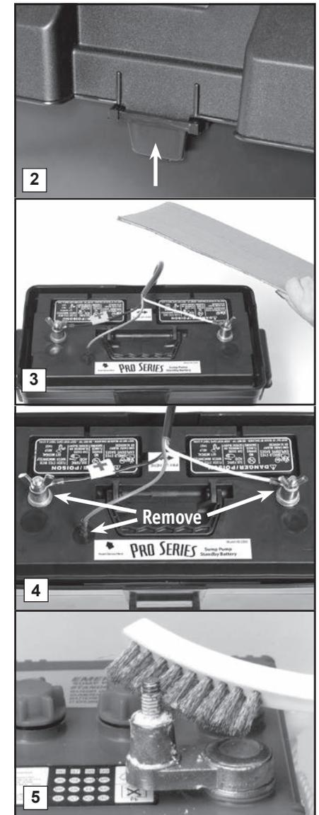
6. Clean any corrosion off of the ring connectors on the ends of the battery wires. Use a stiff brush or sandpaper. **DO NOT** apply corrosion resisting sprays or pads to the terminal rings or posts after you have cleaned them, since this could prevent the battery from charging properly.
