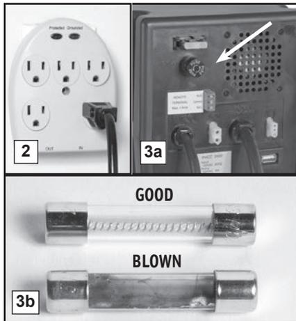
clockwise. Replace the fuse by pushing it in and turning clockwise. (b) If the wires are burned and broken, replace the fuse with a 5 amp glass barrel fuse, commonly found at hardware stores and auto supply stores. Plug in the control unit. (You should provide additional protection for the control unit by using a surge protector.) If the fuse blows again, call Glentronics technical support at 800-991-0466.
