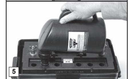
If distilled water is not available, tap water with a low mineral content may be used. Well water is not recommended. **NEVER ADD MORE ACID.**
