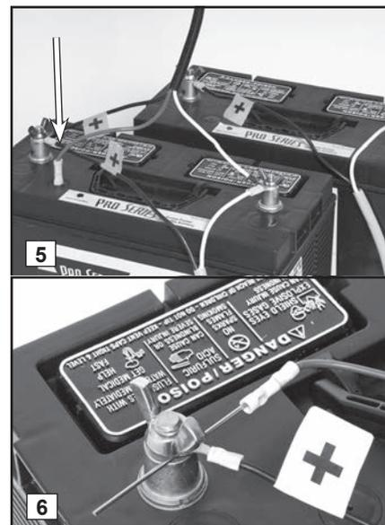
8. If you are connecting two batteries to the system, before you replace the wing nuts, connect the additional cable to the two batteries...the BLACK wires to the POSITIVE (+) posts and the WHITE wires to the NEGATIVE (-) posts of each battery. **NEVER** attach one end of the positive wire to the positive post and the other end of the positive wire to the negative post on the other battery.
