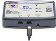
2A-2. Connect the standard USB end into the USB port on the backup sump pump controller
