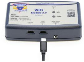
2B-2. Connect the USB end into the USB port on the pump controller
