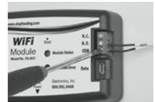
4. On the same end of the remote terminal cable, attach the cable end labeled 'COM' to the Common port labeled 'COM' on the right side of the WiFi module. Turn the screw clockwise to secure the wire.
