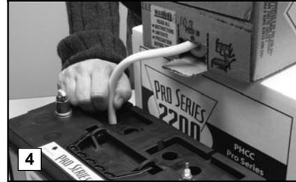
*then go back and top off each cell equally. It is important to have all the cells filled equally or the battery will not operate properly.* The acid should reach a level about 1/4" below the cap ring as shown in Diagram B on the previous page. **DO NOT OVERFILL THE BATTERY** (See Diagram B).
