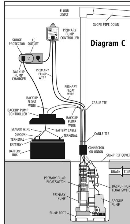
battery cap that is 2nd from the POSITIVE (+) post with the battery cap that is provided in the Pro Series package. An arrow on the top of the battery marks this position. There are two holes in the battery cap. Insert the fluid sensor in the hole that is off-center on the top of the cap. *Do not glue the sensor into the cap.*
