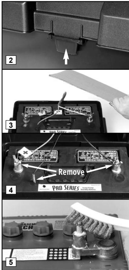
5. Clean the battery posts with a battery terminal cleaner or a wire brush.
