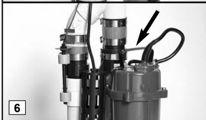
5. Slowly loosen the no hub coupling on the top of the combination pump assembly to separate the pipes. The water trapped in the pipe will pour out into the sump as the no hub coupling is loosened.
