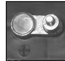
POSITIVE POST HAS LARGER DIAMETER
