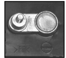
NEGATIVE POST HAS SMALLER DIAMETER
