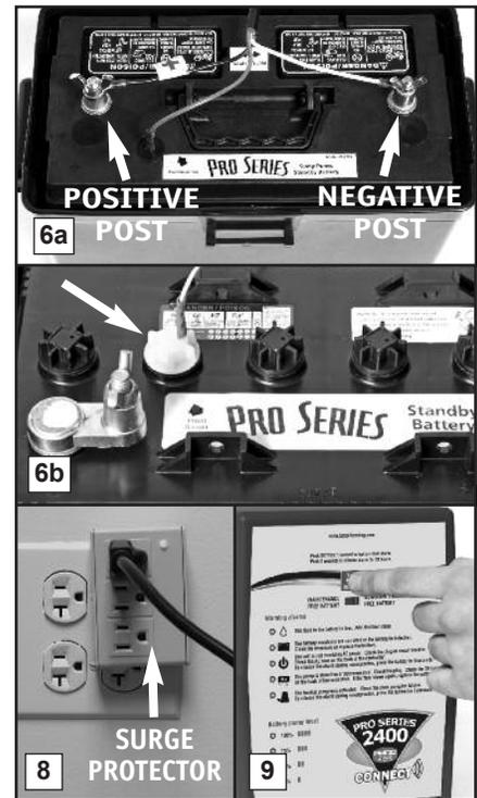
6. Replace the battery caps. Replace the fluid sensor in the hole on the top of the battery or in the yellow battery cap, depending on which battery you own. Be sure the fluid sensor is positioned in the second cell from the positive post. The hole is marked with an arrow. Replace the battery cables...the WHITE wire to the NEGATIVE (-) post, and the BLACK wire to the POSITIVE (+) post. Replace the wing nuts and tighten.
