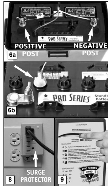
6. Replace the battery caps. Replace the fluid sensor in the hole on the top of the battery or in the yellow battery cap, depending on which battery you own. Be sure the fluid sensor is positioned in the second cell from the positive post. The hole is marked with an arrow. Replace the battery cables...the WHITE wire to the NEGATIVE (-) post, and the BLACK wire to the POSITIVE (+) post. Replace the wing nuts and tighten.
