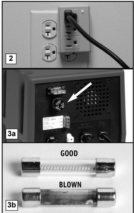
1. If the power is on in the rest of the house, check the home circuit breaker or fuse box for failure, and correct the problem.
