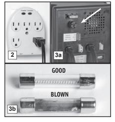
clockwise. Replace the fuse by pushing it in and turning clockwise. (b) If the wires are burned and broken, replace the fuse with a 5 amp glass barrel fuse, commonly found at hardware stores and auto supply stores. Plug in the control unit. (You should provide additional protection for the control unit by using a surge protector.) If the fuse blows again, call Glentronics technical support at 800-991-0466.
