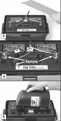
If distilled water is not available, tap water with a low mineral content may be used. Well water is <u>not</u> recommended. **NEVER ADD MORE ACID.**
