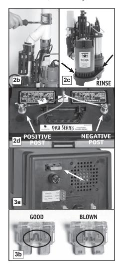
battery...the WHITE wire to the NEGATIVE (-) post, and then the BLACK wire to the POSITIVE (+) post. Tighten the wing nuts on the battery posts. (e) Plug the control unit back into the wall outlet.
