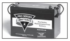
This backup system will also accommodate a maintenance-free battery, eliminating the need to fill the battery. The fluid sensor is not needed with this battery. However, you **MUST** attach the fluid sensor to the positive post of the battery to silence the fluid alarm. Slide the switch on the front of the controller panel to the type of battery being used with the system.
