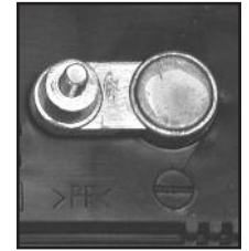
NEGATIVE POST HAS SMALLER DIAMETER
