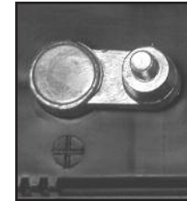
POSITIVE POST HAS LARGER DIAMETER
