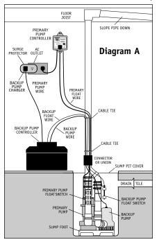
pit is not clean, remove as much of the debris as possible. The pumps are attached to a sump foot (stand) to raise them above any debris.
