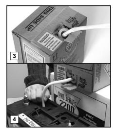
then go back and top off each cell equally. It is important to have all the cells filled equally or the battery will not operate properly. The acid should reach a level about 1/4" below the cap ring as shown in Diagram B on the previous page. DO NOT OVERFILL THE BATTERY (See Diagram B).
