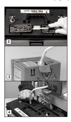
A newly filled battery will sometimes require additional acid after about 20 minutes. Reexamine the fill level, and add additional acid if necessary. The battery acid may bubble at this time and give off a sulfur-like smell, but this is normal. After the battery has been filled, press the caps securely on the top of the battery.
