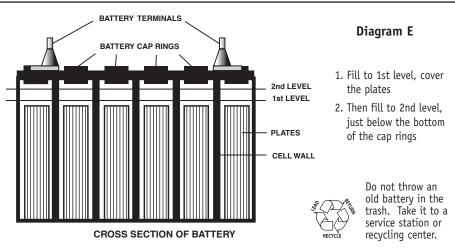
time and give off a sulfur-like smell, but this is normal. After the battery has been filled, screw the six (6) caps securely on the top of the battery.
