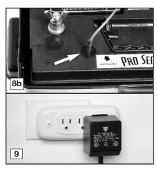
fluid sensor in the top of the battery next to the arrow.
