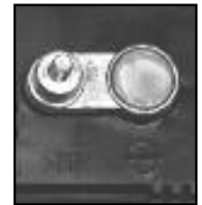
NEGATIVE POST HAS SMALLER DIAMETER
