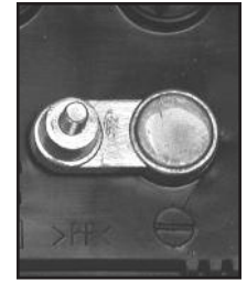
NEGATIVE POST HAS SMALLER DIAMETER
